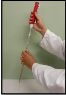
1. Carefully insert your pipette into the cone while applying light pressure.
