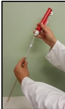
7. Once you've finished your work, pull the pipette gently to remove it from the cone.
