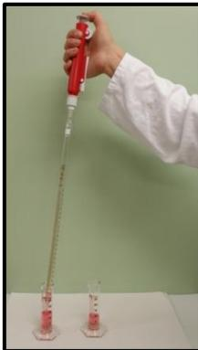
6. Pressing down the piston can release the liquid as well.
