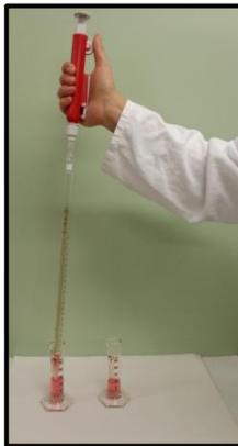
5. To release the liquid more precisely, i.e. line by line, turn back the wheel.
