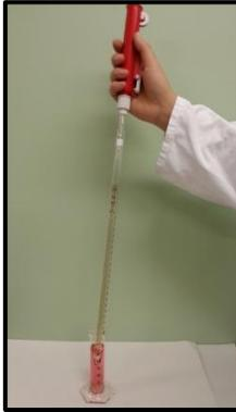
2. Put top of the pipette into the liquid.
